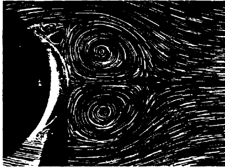
Figure 24. Experimental visualization of Bouard and Coutanceau 11 for Re = 3000 at T = 5
